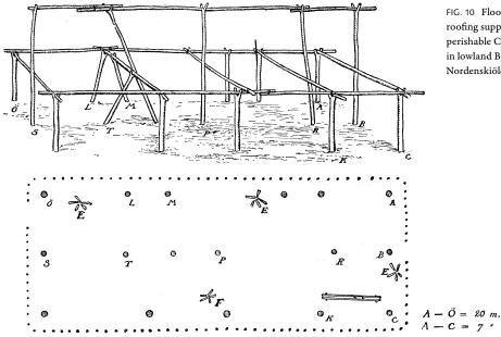
FIG. 10 Floorplan and roofing support system of a perishable Chacobo maloca in lowland Bolivia (after Nordenskiöld 1922)
