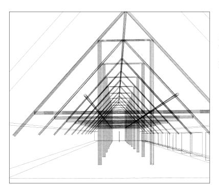
FIG. 7 Hypothetical reconstruction of the kallanka roofing system (Hypothesis 1) shown in an alternative isometric perspective (drawing by Fernando Terrazas)
